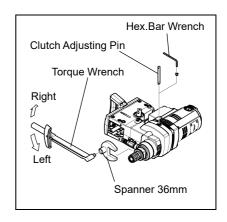
4) After completion of 1) - 3), pull out Clutch Adjusting Pin. Hang Single-ended Wrench 36mm on the Main Shaft and then stick the Main Shaft by a handle of the wrench touching the Pole. Make sure that the Main Shaft is locked. Turn the Motor Switch on for just a moment and make sure that the clutch is slipping without motor locking.
