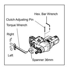
5) After completion of 1) - 4), pull out Clutch Adjusting Pin. Hang Single-ended Wrench 36mm on the Main Shaft and then stick the Main Shaft by a handle of the wrench touching the Pole. Make sure that the Main Shaft is locked. Turn the Motor Switch on for just a moment and make sure that the clutch is slipping without motor locking.
