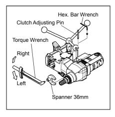
5) After completion of 1) - 4), pull out Clutch Adjusting Pin. Hang Single-ended Wrench 36mm on the Main Shaft and then stick the Main Shaft by a handle of the wrench touching the Pole. Make sure that the Main Shaft is locked. Turn the Motor Switch on for just a moment and make sure that the clutch is slipping without motor locking.
